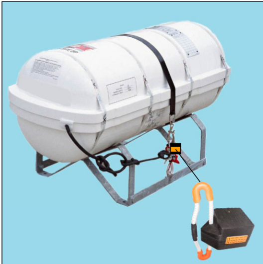
SEAMATE Ve-1 HRU rope connected to the deck
